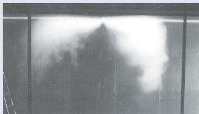
Fig. 1: sin Varyset, \dot{V} = 22 \text{ l/s} ; \Delta t = - 8 \text{ K}
