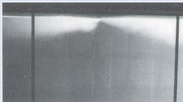
Fig. 5: VSD-1-Varyset, \dot{V} = 44 \text{ l/s} ; \Delta t = - 8 \text{ K}
