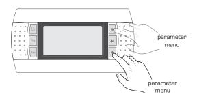
(c) When the desired parameter is displayed, press the ( ) key to enter the parameter. To exit the parameter and go back to the parameter selection mode, press the ( ) key;
