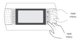
(c) When the desired menu is displayed, press the (v) key to enter the menu. To exit the menu and go back to the menu selection mode, press the (v) key;
