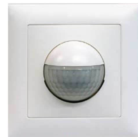
Motion detectors include a PIR sensor (passive infrared) for detecting people in a room, i.e. occupancy. The condition (i.e. if the room is occupied or not) is transmitted to the control system via a volt-free digital output.
