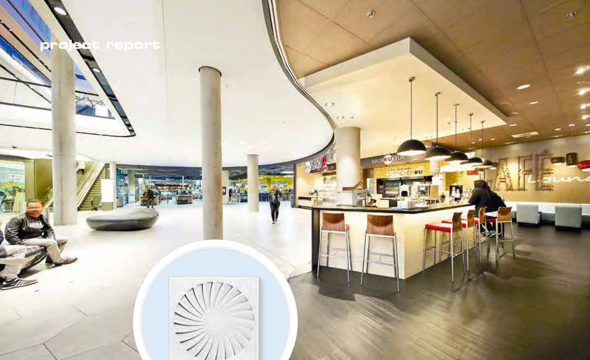
Ceiling diffusers such as TDF SilentAir are ideal for comfort areas due to their low sound power levels.
